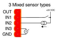
The example above shows 3 different sensors connected to the same input plug-in connector. Input terminal "IN1" is connected to a potential free contact to +24V DC.
