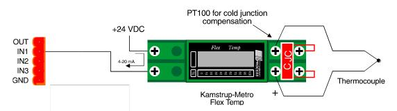
The transmitter snown above works like a current gate. It releases only 4mA at 0°C and 20mA at 100°C.
