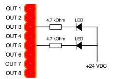
The open collector output "AL.OUT" can be used to signal the appearance of multiple alarms controlling the same output.
