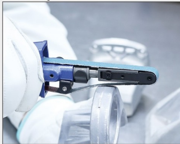
Detail finishing of aluminum material.
