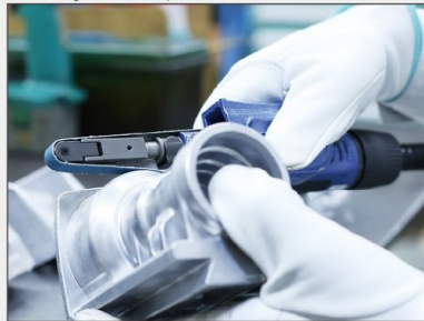
Deburring of die cast parts.
