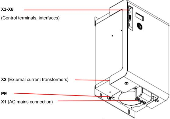
Fig. 30: Position of the electrical connecting terminals ECOsine® active -30/50-xxx-3
