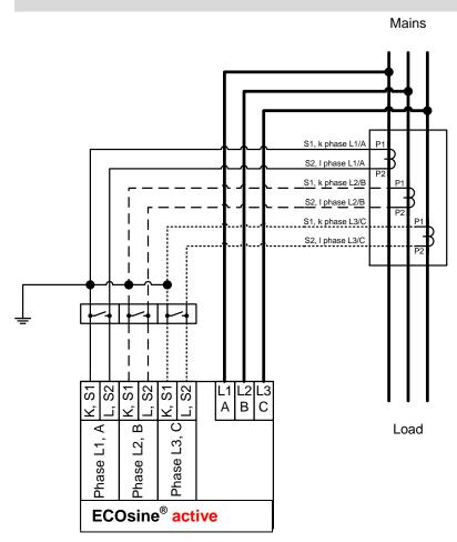
Fig. 55: Grounding of the current transformers (optional)
