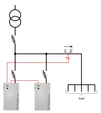
Fig. 53: CT installation on load side for parallel operation of several ECOsine® active devices
