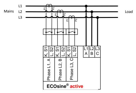
Fig. 41: Connection of 3-wire devices
