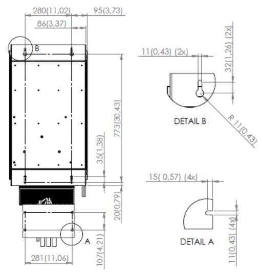
Fig. 19: Drilling template ECOsine  $^{\tiny{\textcircled{\scriptsize 0}}}$  active FN3420-100/120-480-3-GL
