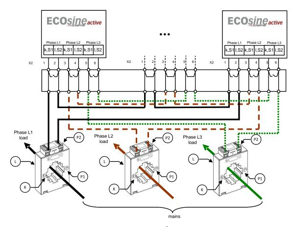
Fig. 52: CT wiring for parallel operation of up to five ECOsine® active devices
