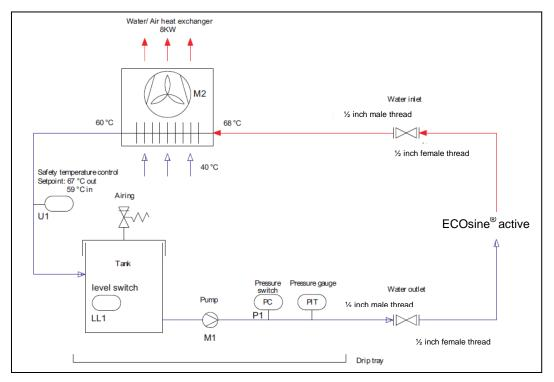
Fig. 5: Cooling system - hydraulic plan
