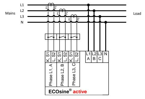
Fig. 42: Connection of 4-wire devices
