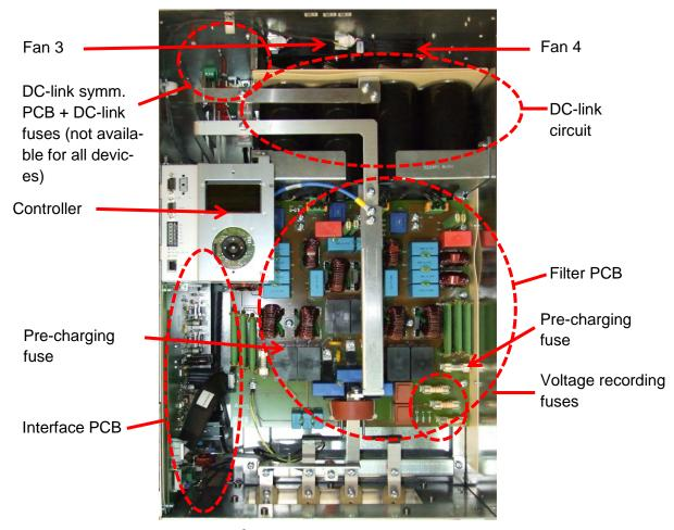
Fig. 46: Component layout plan ECOsine® active FN3430-100/120-400-4
