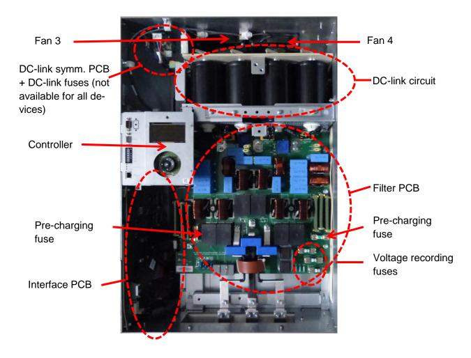
Fig. 45: Component layout plan  $\mathsf{ECOsine}^{\$}$  active  $\mathsf{FN3420\text{-}100/120\text{-}xxx\text{-}3}$
