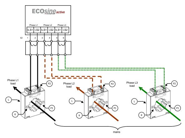
Fig. 49: CT wiring for operation of one ECOsine® active
