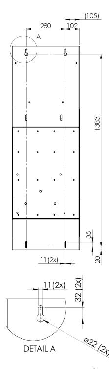
Fig. 21: Drilling template ECOsine® active FN3430-100/120-400-4
