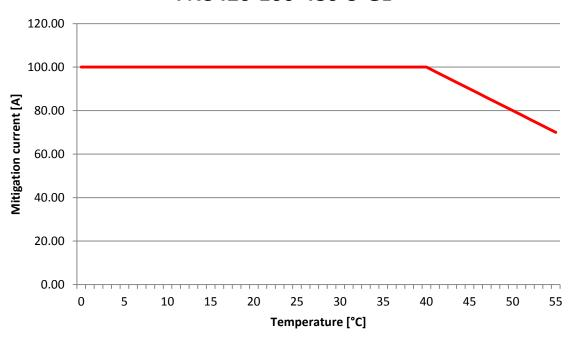
Fig. 80: Derating ECOsine® active FN3420-100-480-3-GL
