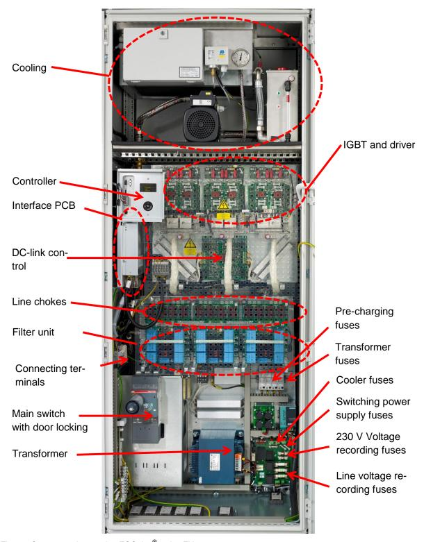
Fig. 48: Component layout plan ECOsine® active FN3420-200-690-3
