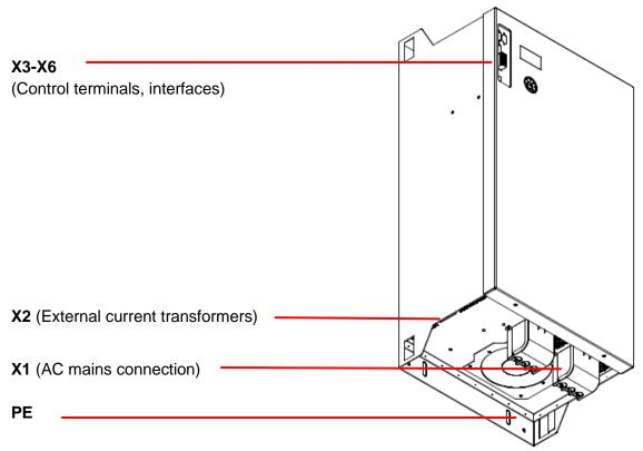
Fig. 32: Position of the electrical connecting terminals ECOsine® active FN3430-30/60-xxx-4
