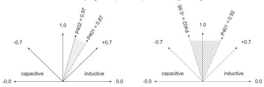
Fig. 68: Example for  $\cos\phi$  control ( $\cos\phi$  on mains side is kept in the hatched target range)
