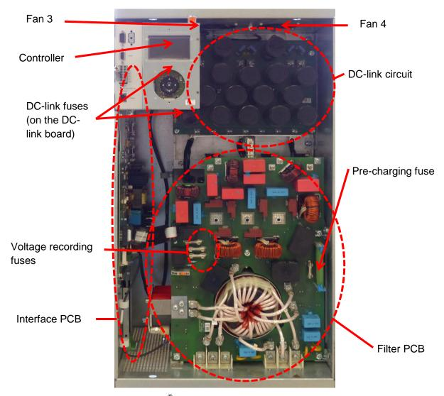
Fig. 44: Component layout plan ECOsine® active FN3420-30/60-xxx-4
