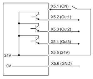
Fig. 62: Functional connection of digital input/outputs
