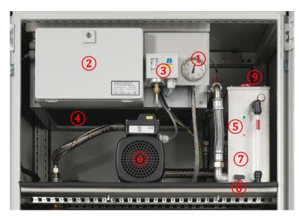
Fig. 4: Cooling system - main components
