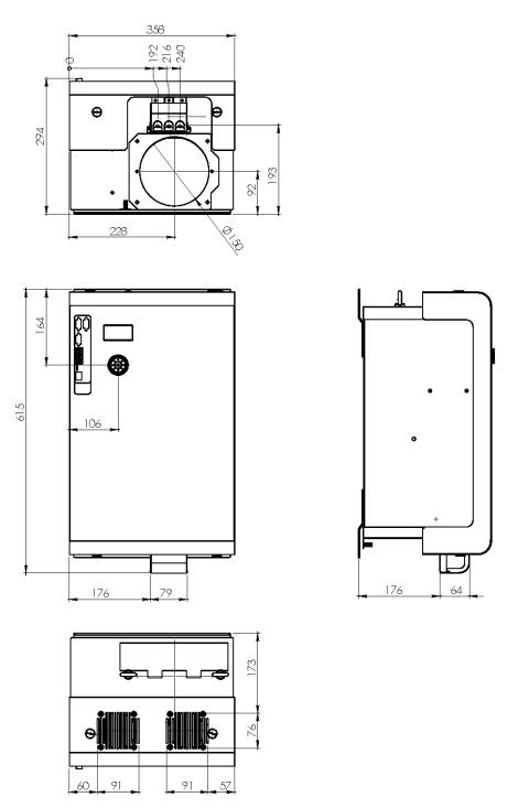
Fig. 12: Dimensional drawings ECOsine® active-030/050-xxx-3
