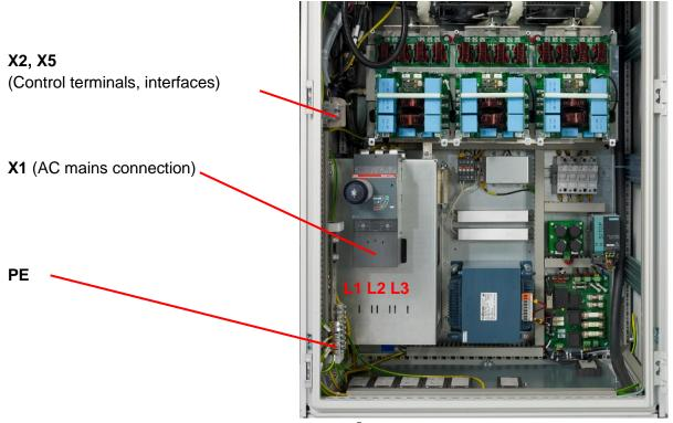
Fig. 40: Position of electrical connecting terminals ECOsine® active FN3420-200-690-3
