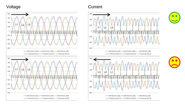
Fig. 56: Checking rotating field of current and voltage
