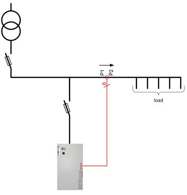
Fig. 50: CT installation on load side for operation of one ECOsine® active
