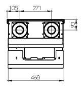
Fig. 20: Dimensional drawings ECOsine® active FN3430-100/120-400-4
