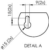
Fig. 13: Drilling template ECOsine® active FN3420-030/050-xxx-3
