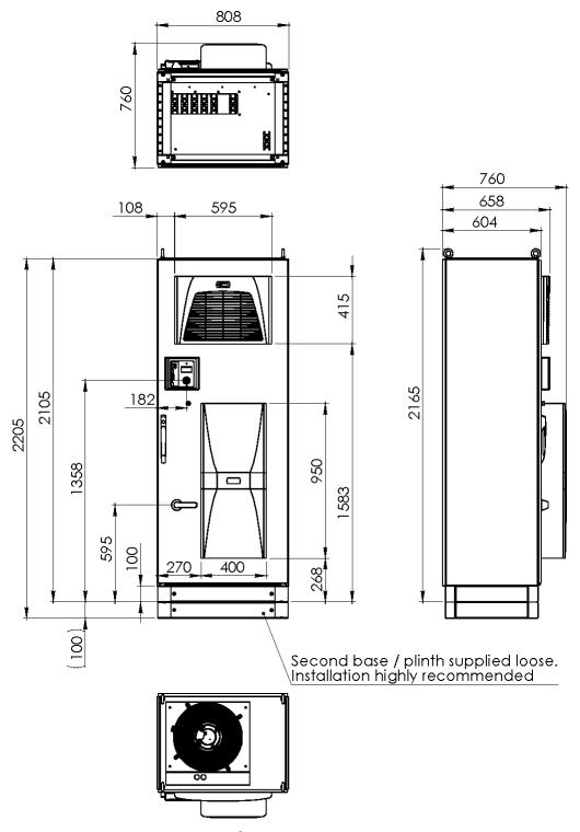
Fig. 22: Dimensional drawings ECOsine® active-200/250/300-480-3 (with mounted base 100 mm)\*
