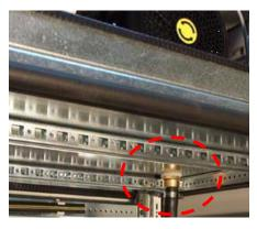
Fig. 9: Drain-tube of water tray
