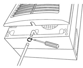
Fig. 11: Connection option for condensate drain at the interior air cooler
