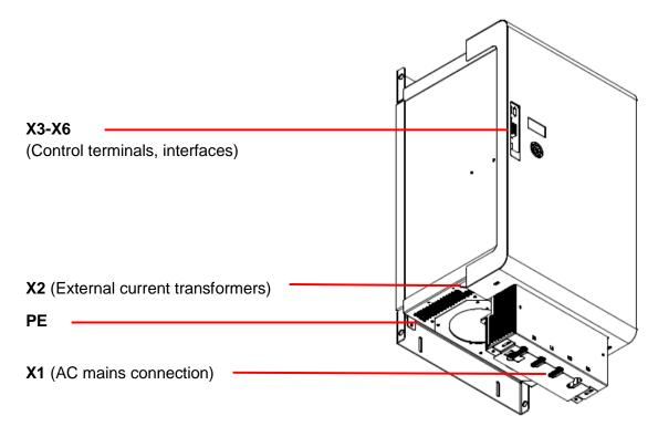
Fig. 34: Position of the electrical connecting terminals ECOsine™ active FN3420-100/120-xxx-3
