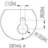
Fig. 15: Drilling template ECOsine® active FN3430-030/060-xxx-4
