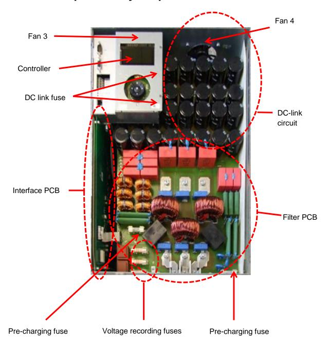
Fig. 43: Component layout plan ECOsine® active FN3420-30/50-xxx-3
