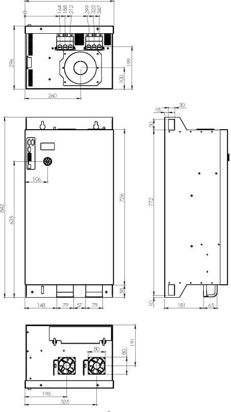
Fig. 14: Dimensional drawings ECOsine® active FN3430-030/060-xxx-4
