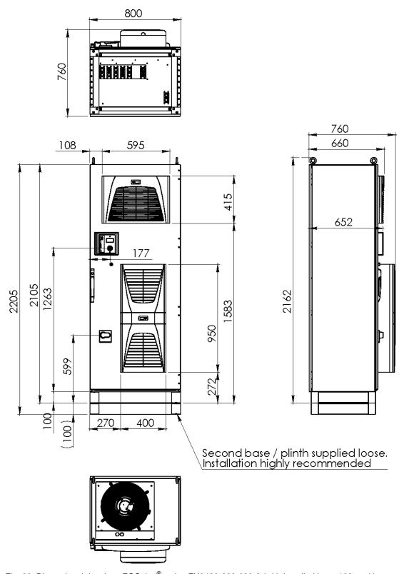
Fig. 26: Dimensional drawings ECOsine® active FN3420-200-690-3 (with installed base 100 mm)\*
