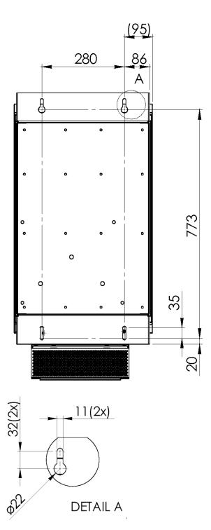
Fig. 17: Drilling template ECOsine® active-100/120-xxx-3
