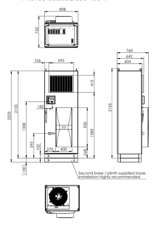
Fig. 24: Dimensional drawings ECOsine® active FN3430-200/250/300-400-4 (with mounted base 100 mm)\*
