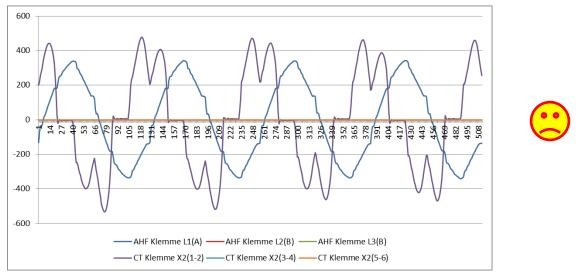
Fig. 60: Current transformers of phase 1 and 3 are interchanged
