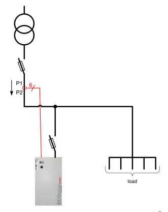
Fig. 51: CT installation on mains side for operation of one ECOsine® active
