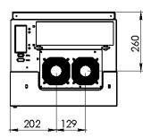
Fig. 16: Dimensional drawings ECOsine® active FN3420-100/120-xxx-3
