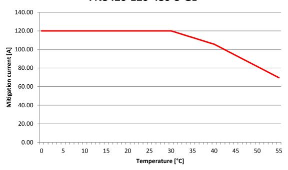
Fig. 83: Derating ECOsine® active FN3420-120-480-3-GL
