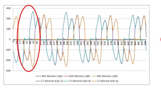
Fig. 59: Current transformer 1 phase-is shifted through 180°.
