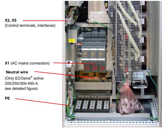
Fig. 38: Position of the electrical connecting terminals ECOsine® active FN34xx-200/250/300-4xx-x
