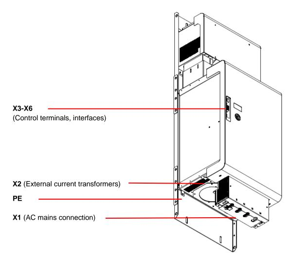
Fig. 36: Position of the electrical connecting terminals  $ECOsine^{\$}$  active FN3430-100/120-400-4
