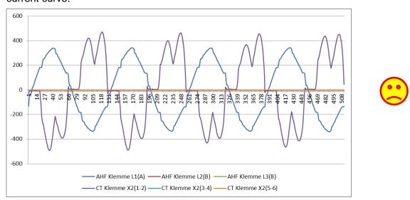
Fig. 58: Phase of current and voltage is shifted through 180°.
