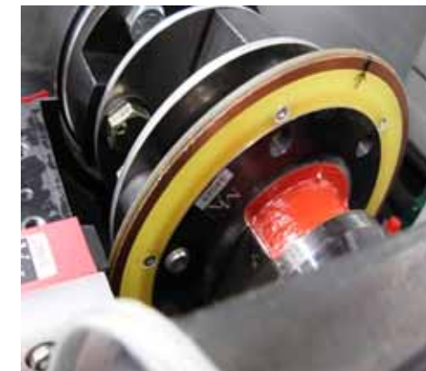
Torque acquisition integrated in coupling
